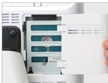
Service Access for Replacing HDD
