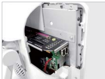
Solid AL Die casting Frame Construction
